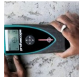
Rebar Mapping & Cover Depth of Concrete
