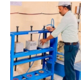
Concrete Depth of Water Penetration
