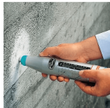
Rebound Hammer Test
